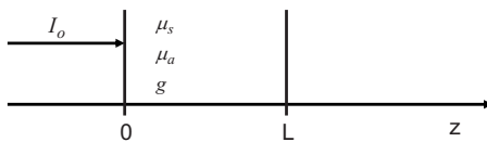
FIG. 3. A cross-sectional view of the model geometry. I_0 : intensity of the incident laser radiation; L : bone thickness; \mu_a : optical absorption coefficient; \mu_s : optical scattering coefficient; g : mean cosine of the scattering angle.
